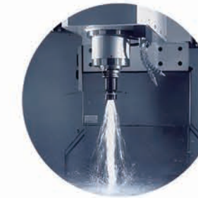
Water flows out from the center of the spindle 主轴中心出水
